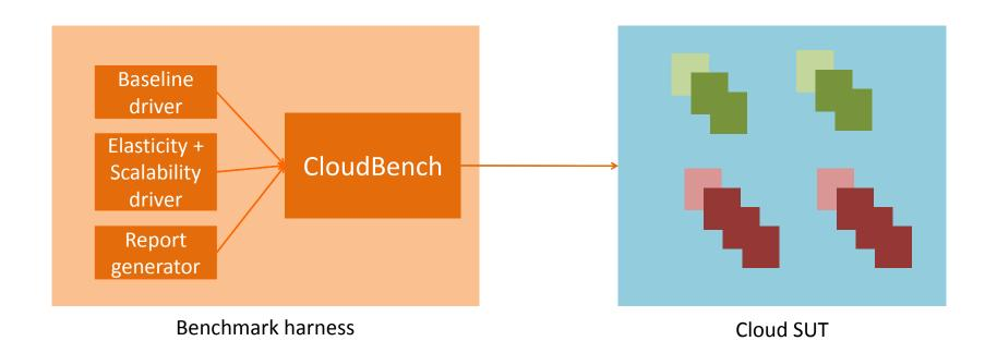
Benchmark harness. It comprises of Cloud Bench (cbtool) and baseline/elasticity drivers, and report generators. cbtool creates application instances in a cloud and collects metrics. cbtool is driven by baseline and scalability driver to execute the baseline and elasticity + scalability phases of the benchmark, respectively.
